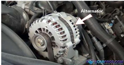
Our car’s alternator is a workhorse. When your engine is running, the alternator charges the battery and supplies power for the vehicle’s electrical systems. There are a lot of electrical accessories and systems in your car, beyond just lights and stereo. Modern cars are loaded with sensors and computers that all require electricity. From lights to GPS systems, the alternator powers it all.
